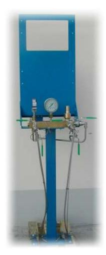
Manually controlled, the FCD22 unit allows to fill cylinders and extinguishers with CO2 transferred from a cryogenic tank. The operator acts on the check valves manually according to the information supplied by the control weighing scale displays. Bundle filling can optionally be obtained on a third weighing appropriate scale
