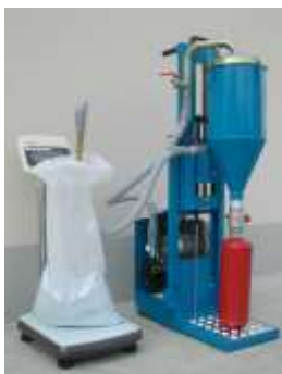
FILLING OF PORTABLE EXTINGUISHER WITH ETW100 SCALE
