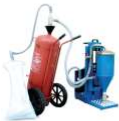
FILLING OF WHEELED EXTINGUISHER WITH "VENTURI" KIT
