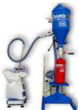
FILLING OF PORTABLE EXTINGUISHER
